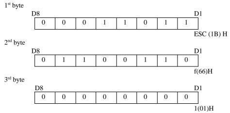
The input of this command feeds the paper to the top of the next page, after printing the data contained in the print buffer.
